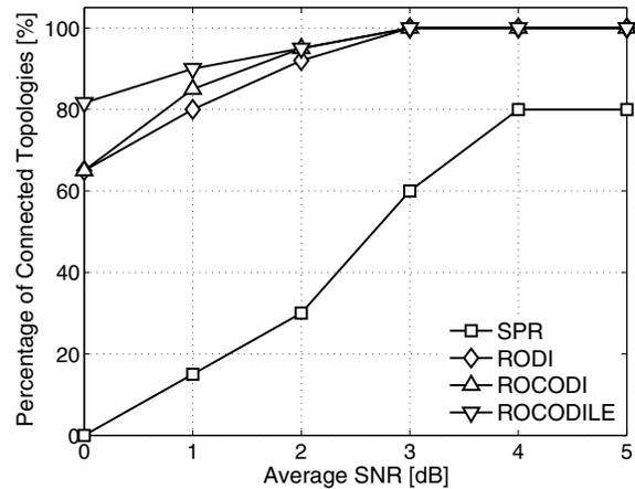
Fig. 6: Connectivity, 25 nodes network
