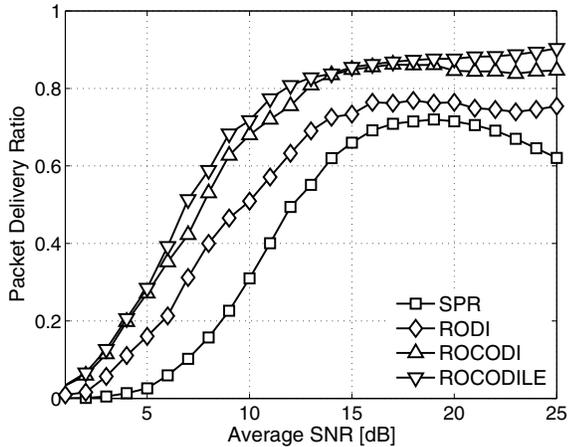
Fig. 5: Packet Delivery Ratio vs SNR, random topology
