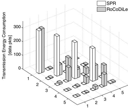
Fig. 3: Transmission energy consumption, grid topology. Source node is located at (1,1) while destination node is at (5,5)
