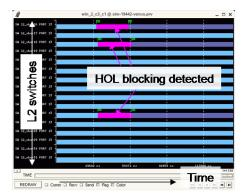
Figure 5: 256-way WRF pattern; HOL blocking on L2 switch ports.
