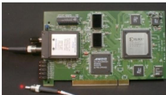
Figure 1: Prototype of the reconfigurable optical network adapter
