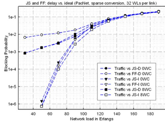
Fig.8. Blocking performance of PacNet
