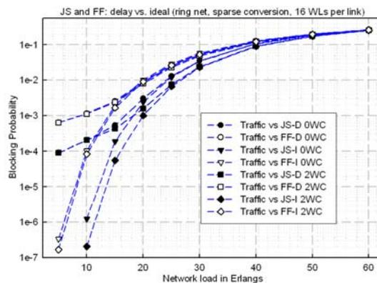
Fig.7. Blocking performance of 12-node ring
