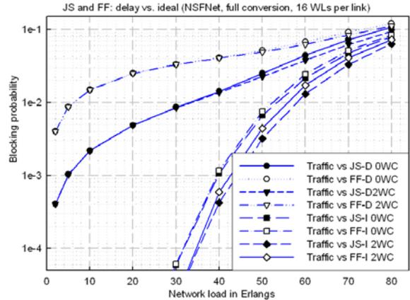
Fig.9. Blocking performance of NSFNet
