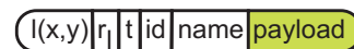
Figure 2: Structure of a data item consisting of a position l , a dissemination radius r_l , a timestamp t , a unique creator id , a name and the payload.
