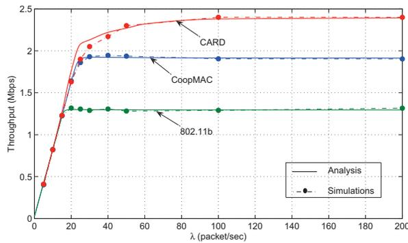
Figure 4: Throughput vs. offered load,  $L=1024$  bytes.
