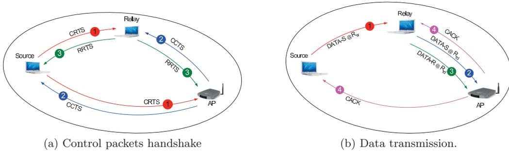
Figure 2: Access mechanism of CARD protocol.
