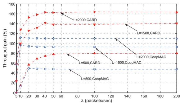
Figure 6: Throughput gain vs. offered load,  $N=30$  nodes.
