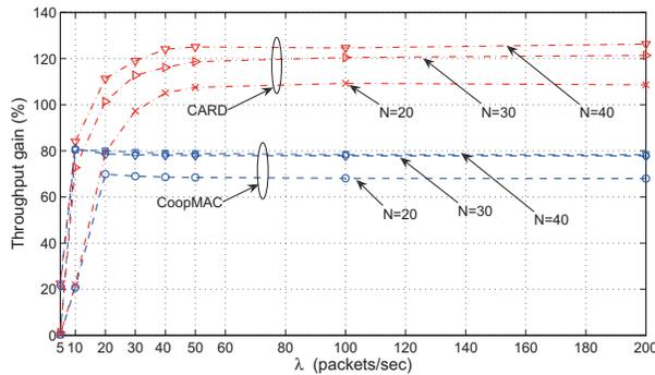
Figure 5: Throughput gain vs. offered load,  $L=1024$  bytes nodes.
