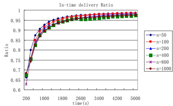
Figure 8. In-time delivery ratio as a function of time under different swarming scales
