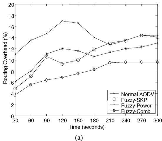
**Figure 5** Routing overhead comparison: (a) 25 nodes; (b) 35 nodes and (c) percentage of improvement than the normal AODV (continued)
