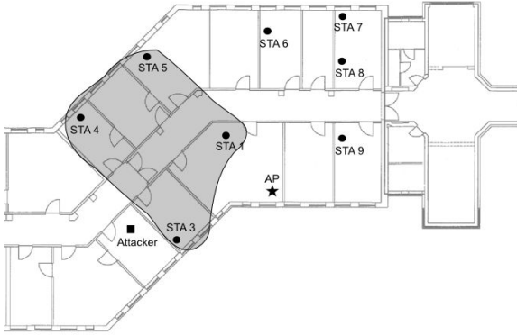
Figure 5: Attack containment: the attacker is successful only in blocking certain regions within its proximity like the region \{1, 3, 4, 5\} . All other regions were still unused and legitimate clients were able to join from them.
