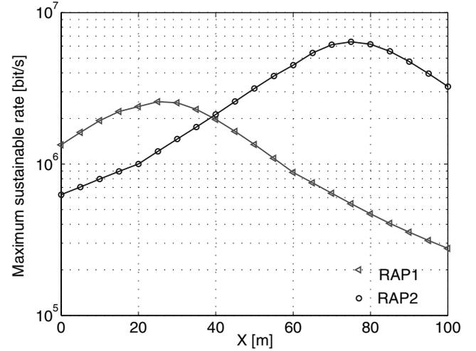
Figure 10. Downlink sustainable rates as functions of the new MT's location.
