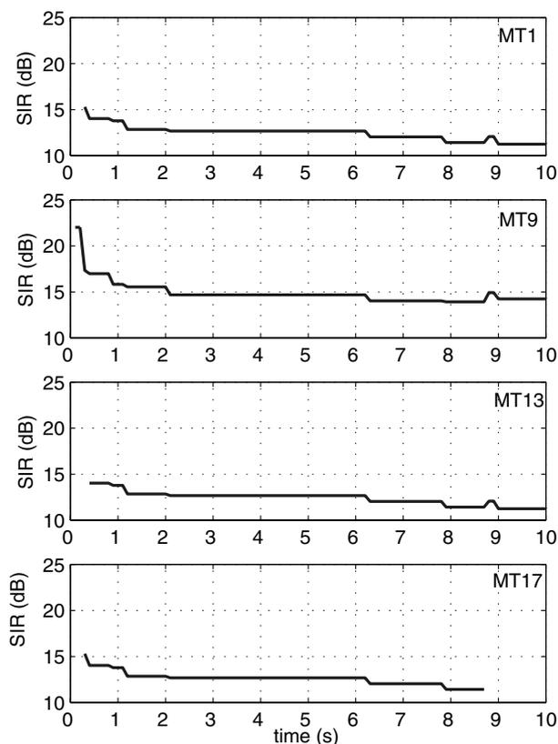
Figure 13. Time evolution of SIR levels with interference weight  $a = 100$ .
