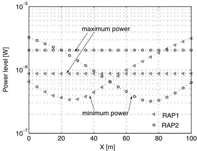
Figure 9. Downlink power levels as functions of the new MT's location.
