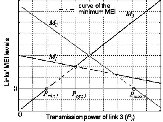
Figure 2. Case of three links: MEI levels as a function of the entering link's transmission power.
