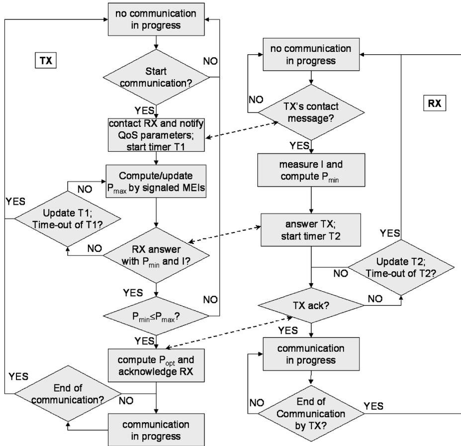
Figure 3. Flow charts of the operations performed at the Transmitter (TX) and the Receiver (RX).
