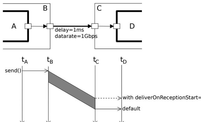
Figure 4.3: Packet transmission
