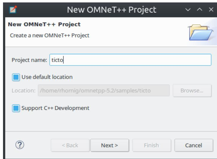
Fig. 5.2: Setting project name and enabling C++ support
